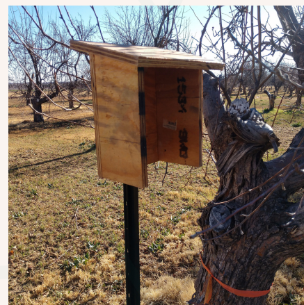
HOUSING FOR DATALOGGER IN ORCHARD FIRE BLIGHT TREATMENT STUDY
